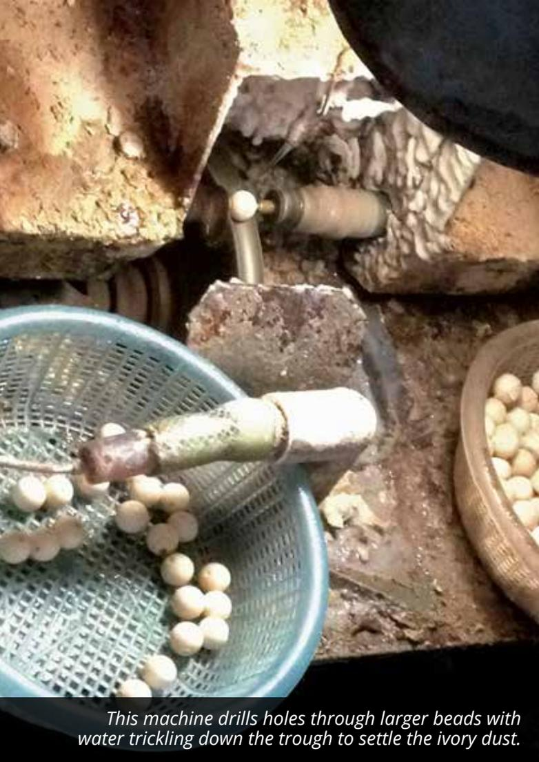
*This machine drills holes through larger beads with water trickling down the trough to settle the ivory dust.*
