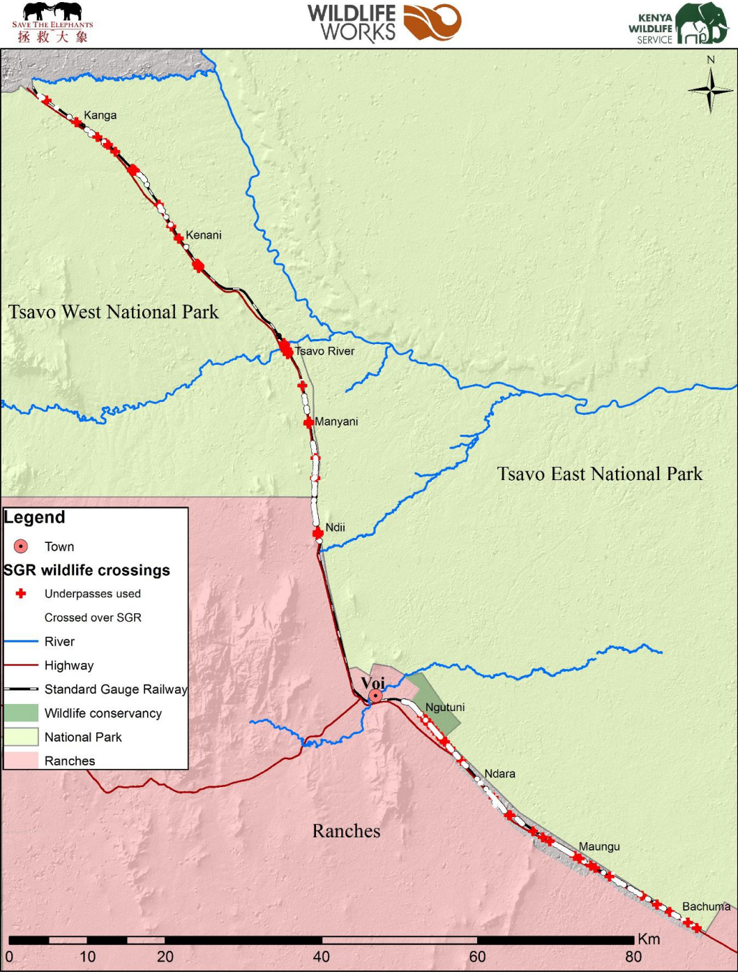
Figure 7: An overall map showing wildlife crossing points along the SGR from Bachuma to Mtito Andei. The red cross signs are areas where wildlife crossed the SGR using a designated underpass, a bridge or a culvert. The white dots are areas where wildlife species were recorded as having climbed over the SGR embankment.
