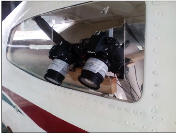
Figure 2. Camera installation in the Cessna 210 aircraft, right side cameras, survey MU4 (April 2016), with cameras angled at 45° through the open 'clear-vision-panels'. The main right-side camera is the further camera (Nikon D3200, 24 MP), but in MU4 an additional camera pair was added for testing (Nikon D810, 34 MP), here the nearer camera (tests not reported here). The system was duplicated on the left side of the aircraft.
