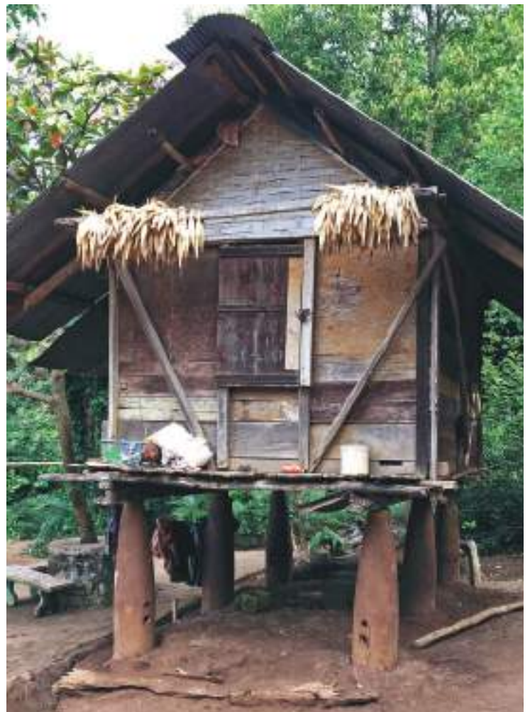
These two rice stores in private gardens in Huay Xai are supported by stilts made of old bomb cases that were dropped by US aeroplanes during the Secret War.
