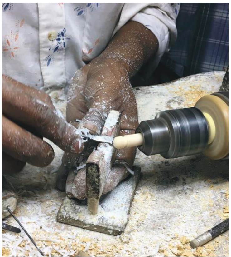
The ivory carver shapes the bead with a wide flat chisel.
