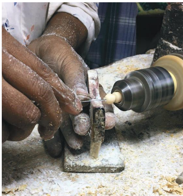
Beads are cut from a solid tube of ivory with a tiny hole made in the middle for the string.
